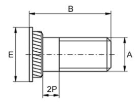
For plate thickness, min = 1.5 Head diameter E = 8 Hole diameter +0.1 = 6.4 Length B = 15 Male thread A = M5x0,8 Min distance to edge = 3.3
